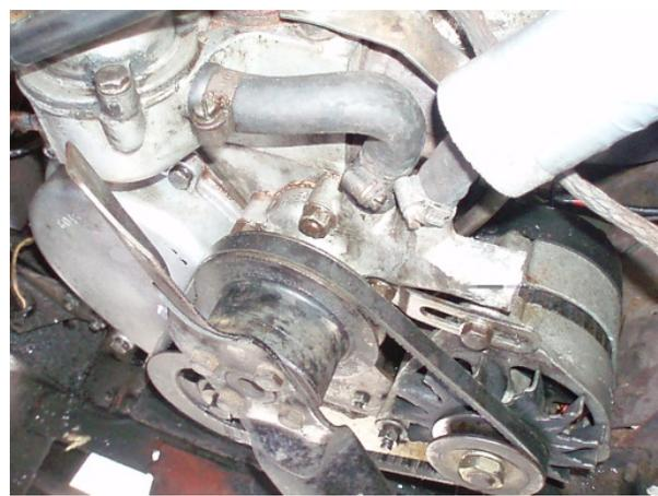
Observant enthusiasts will spot the redundant mechanical fuel pump, must remember to get a blanking plate and remove the old pump, I often wonder how much energy is wasted cranking its operating lever up and
