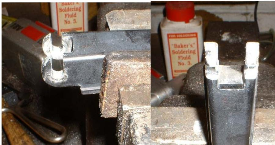
A test fit showed the centre section of the other hinge between the outer leg parts needed a slight amount filed off, allowing the hinge parts to latch together freely.
