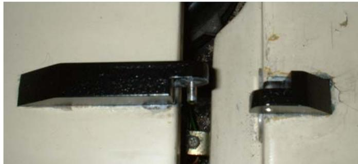
As can be seen they consist of “half hinges” with pivot pin and are now of solid bar construction instead of cast construction. I still prefer to be able to “whip off” the bonnet when required, for easy access to engine bay.
