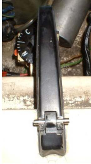
Testing again after showed the hinge to latch together in vertical position and to drop freely to the locking position. Pin width was then cut off either side to match the hinge profile and cleaned up with a file.
