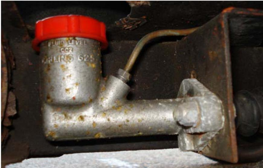
Thanks for the pictures. I see that the body bears the markings "CC2" and "G25". I think that G25 is the casting type and any replacement Girling master cylinder of the correct size should carry this reference. Be aware that the bore size could be different though, because there was nothing to stop Girling from boring out the same standard casting with different bore sizes.
