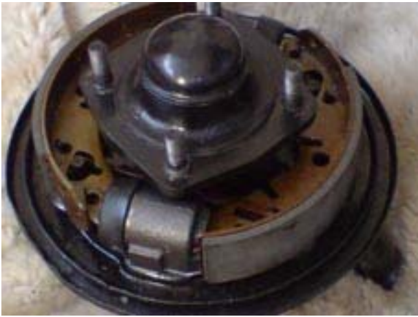
The re-furbished front brakes – inside,
