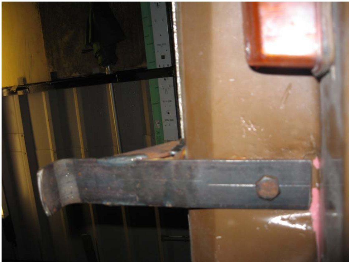
Two shots of the excellent body lifting brackets designed by Brian Revill. Brian might be prepared to make more sets if required. Contact the Registrar in the first instance.
