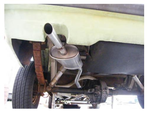
Within 3 days I received the exhaust, very well packed, all-in good order. The exhaust came in two pieces, downpipe complete with bracket for attachment to the engine flange, and second half with silencer.
