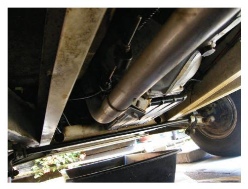
My Kitten is a left hand drive one, so I have the clutch cable and clutch operation at the left side, where the exhaust passes. Because of the clutch cable I had to attach the bracket to the lowest stud on the engine flange. Everything kept clear of the exhaust, so also for left hand drive it is a straight fit.
