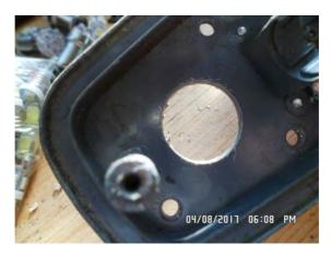
I just drilled out the rivets holding the reflectors, then a 22mm hole. I also removed the old busbars that connected to the bulbs.
