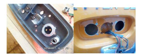
I removed the factory plastic "rawplugs" and replaced them with 4mm "Rivnuts". Then just drilled a pair of matching holes to clear the bulb holders.
