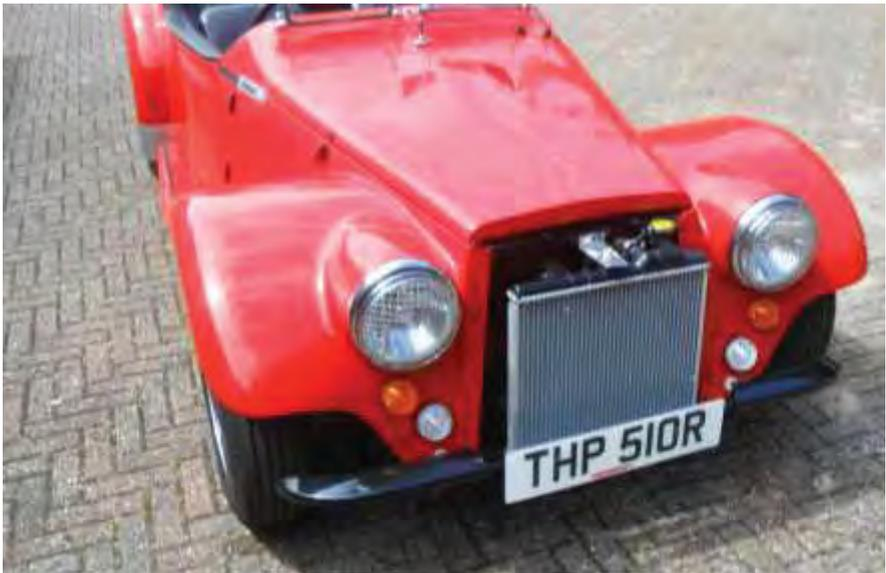
One piece of box section frame was removed making space for a pair of base brackets, fabricated with holes to accept the plastic positioning lugs. With the top secured by a similar steel plate, longer hoses were sourced along with fresh alloy tubing. Plumbed in, fresh coolant, plus a final oil change, and four months behind schedule she is done, and runs like a dream; its only taken three and a half years since I first found it languishing at the back of Professor Anthony Stevens unit in Kent.
