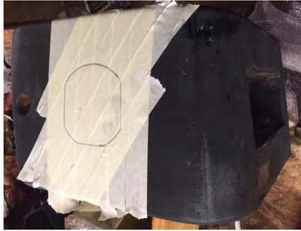
Now check the socket fits. It might need minor trimming to make it fit. Holding the socket in, use a small drill bit (roughly 2.5mm) and drill the 4 retaining screw holes and pop in some screws. I used stainless steel as being on the outside of the Fox, if I need to remove it, hopefully they won't have rotted away!
