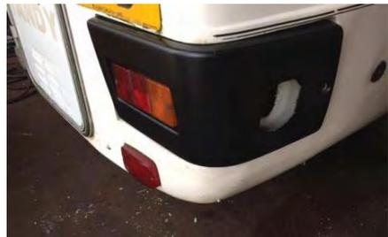
Now with the bumper paint dry, bolt the bumper back onto the Tandy. The rubber flap which was glued on before can now be rolled up to the inside of the bumper. Doing this will create a 'roof' over the socket on the inside of the bumper. Any water which comes down the body
