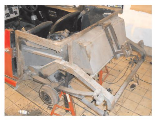
One nice part of the design is the front wing and tread plate under the doors is one complete panel supported by out-riggers from the chassis itself; unfortunately these were all 'wafer' thin and crumbled to the touch.
