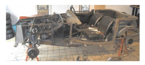
The original chassis drawings show just how heavily modified ours was compared with how it began life. The basis was from a Reliant Kitten, and the original metal was in great shape, with just light surface corrosion, although anything attached to it was made from 1" box section tubing, and that was not so clever.
