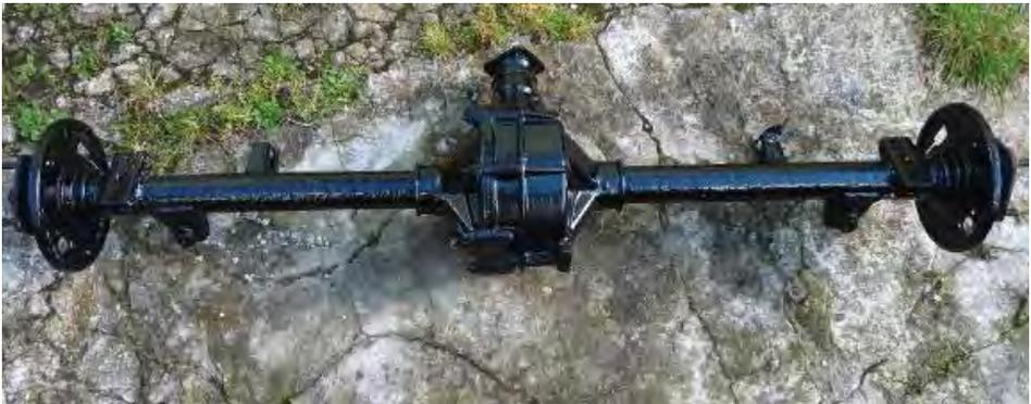
The front seal on the rear axle is leaking so this will require replacing. Now came a shock. It was a three wheeler axle. To cut a long story short, I was unable to remove the hubs and back plates to replace with Kitten ones and so have had to rebuild as is. I bought new cylinders but will now wait until better weather and warmer days before the enjoyable task of reassembly.
