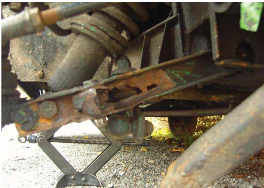
The problem of course was not so much the holes in the lower wishbone, but the failure of the tie rod! (strut if you will).
