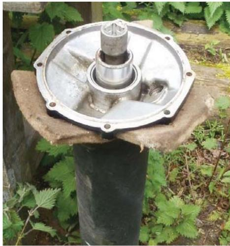
You will need to heat the casing with a blowlamp first to get the alloy casing to expand enough to release the tubes.
