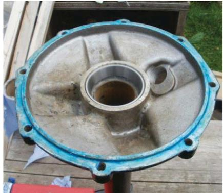
Smear the casing mating surfaces with gasket compound & reunite the 2 halves.
